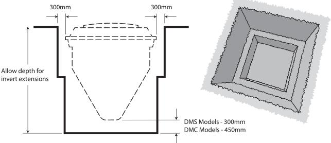
A square stepped excavation may be used due to the physical shape of the Diamond plant. Allow adequate clearance for all pipes and any other connections the unit.
