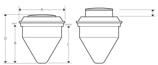
DMC turret extensions are available in 100mm increments up to a maximum of 1200mm
