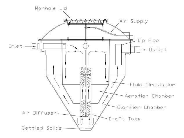
The sectional drawing above shows a typical DMS treatment tank but the larger DMC models work on exactly the same principle. To calculate the trench size for the Diamond plant to be installed refer to the size chart and groundworks diagram on page 6 & 9.
